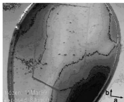
Figure 4. A plate-like crystal of \text{Ca}^{2+} -ATPase mounted in a nylon loop. The width of the crystals measures \sim 400 \mu\text{m} ; the thickness is approximately 20 \mu\text{m} . Note that the specimen was examined with laboratory source and stored in liquid nitrogen for more than one year prior to the diffraction experiment at BL41XU and that no severe frosting was observed.
