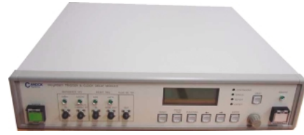
Fig. 7 Photograph of precise timing delay unit. The unit is composed of a continuous phase shifter of 508.58 MHz RF signal, frequency dividers, and digital memories to control the phase or timing delay.
