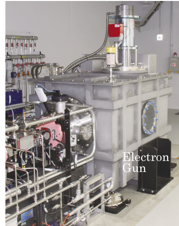
Fig. 2 Outlook of the 500 kV, CeB 6 thermionic electron gun.
