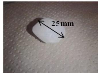
Fig. 3 (Color online) A natural gas hydrate pellet at 253 K under atmospheric pressure.
