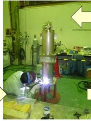
TIG weld of He Jacket at CFF
